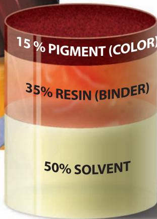
Paint consists of three parts: pigment, resin and solvent. After high performance finishes are factory applied, the coated product is baked, and the solvents are released and incinerated leaving the pigments and resins on the substrate.
